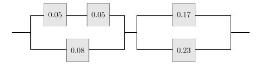
**Note:** Each gray box is a device. It fails with the probability written in the box and all devices fail independently. The circuit works only if you can go from left to right along the wires through working devices without passing a failed device.
